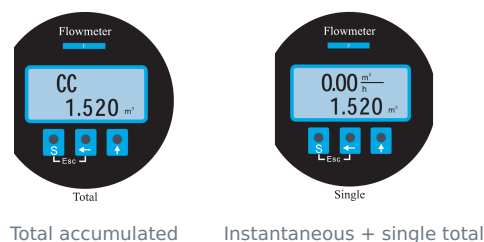
Fig. 4 — Register display interfaces. The single-cycle total is reset at the instrument.
